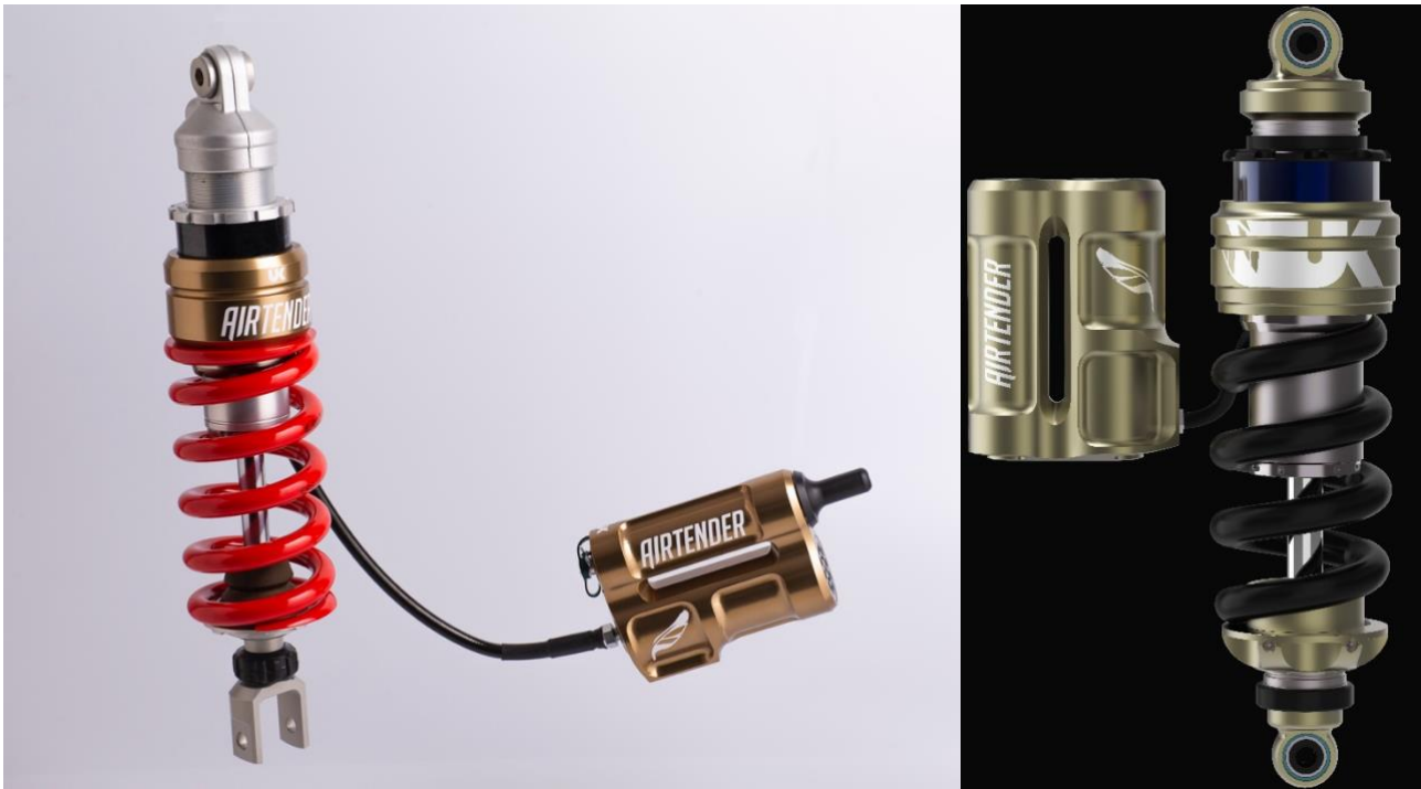
Fig. 1: Shock absorbers equipped with AirTender. The hydropneumatic spring is in series with the coil one.
